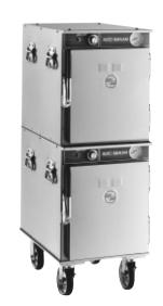
Clearance: Minimum clearances are required for proper air ventilation including 3-inches (76mm) at the back, 2-inches (51mm) at the top, and 1-inch (25mm) at both sides. On site venting for proper airflow must also be provided for built-in installations.
